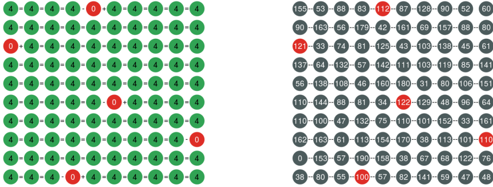
Figure 7.7 DR_5 data rate sequence (left) and TR_5 time sequence (right) for link disconnection
